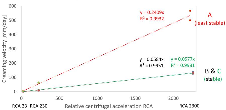
All three emulsions show a linear dependance of their creaming velocity on RCA. The calculation of the creaming velocity at gravity (RCA=1) is possible by linear regression.
