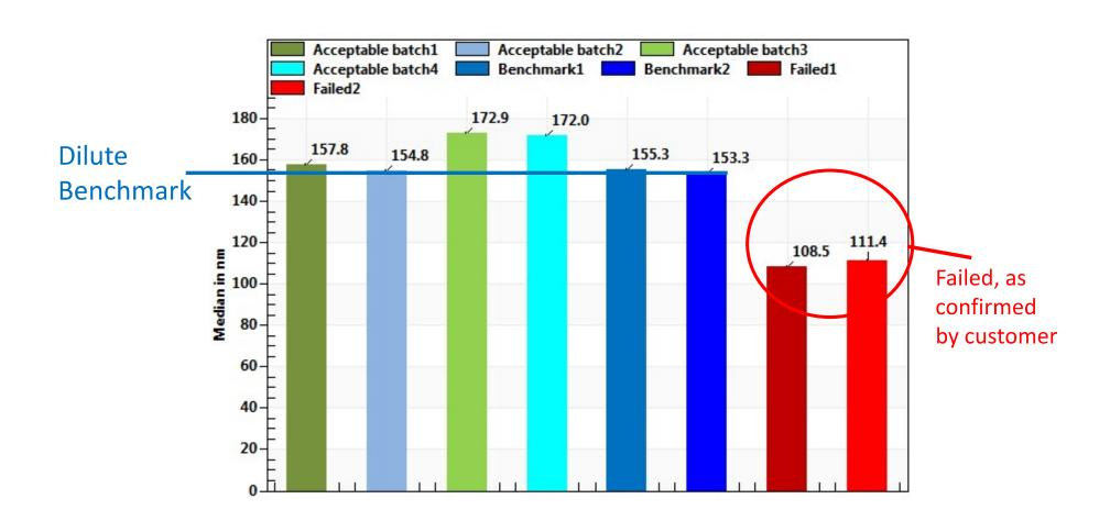
Droplet size distributions of creaming particles, calculated with customer's material data, are in agreement with the results from other particle sizing methods. Dilution for LUMiSizer 1:20 (m/m).
