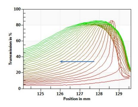
38 h real-time separation at gravity, RT, every 10<sup>th</sup> profile shown.
