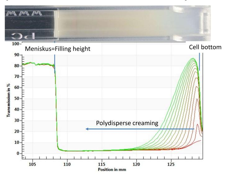
125 minutes accelerated separation at RCA 2300, 25 °C, every 10<sup>th</sup> profile shown, 870 nm, photo after 125 min.
